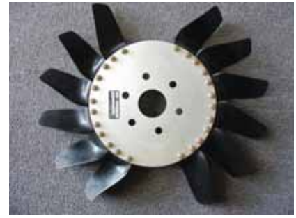
From the original fan blade, a Perceptron laser scanner generated a 3-D point cloud that was converted into math surfaces using Geomagic Studio software. A new injection mold was created to manufacture the blades from glass-filled acetal.
