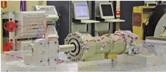
Belgian firm SABCA is using LMS Test.Lab software to conduct qualification tests of thrust vector control systems (shown) to be used in the European Space Agency's VEGA launcher.
