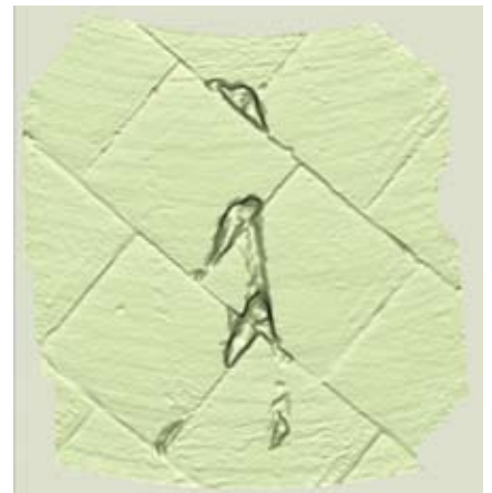
Shown is a digital reconstruction of tile damage automatically created in Geomagic Studio based on data captured from a Neptec scanner.
