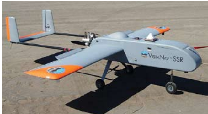
The VistaNav-SSR (smart surveillance and reconnaissance) is a complete, high-performance unmanned aircraft system that includes a ground control station integrated with 3-D synthetic vision and a small UAV. UAV technology is one of the areas expected to benefit from the multicore technology used in next-gen gaming devices.
