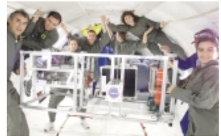
*The AMDS experiment was run in the KC-135 airborne test laboratory that replicates the effects of micro-gravity for on-board experimentation.*
