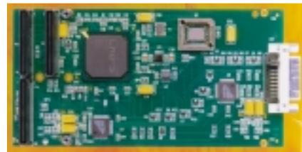
of embedded SDRAM, the new PMC is able to support 83 MHz operation. The PMC-DGX can seamlessly replace the CPCIGx and GTX8 graphics boards.
