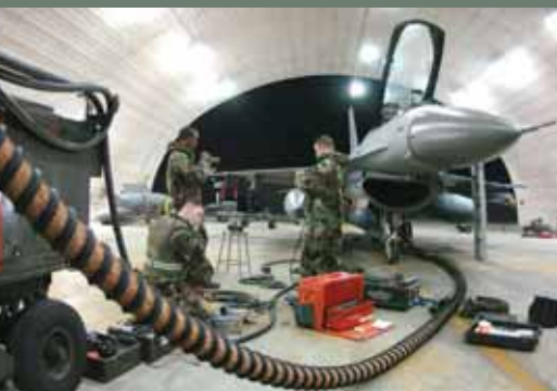
Airmen check F16 flight-control air data system
