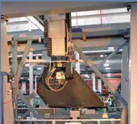
Gantry trim and drill machine for precision high-speed drilling and trimming.
