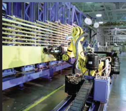
Reconfigurable multi-axis robotic drilling/tacking cell for determinate assembly.
