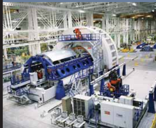
Broetje auto riveter drills and installs fasteners common to skins and substructure.
