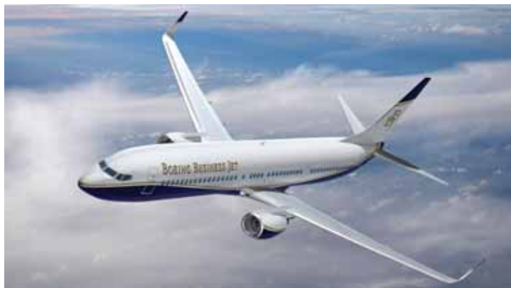
With up to five auxiliary fuel tanks, the BBJ 3 will have a range of 4765 nmi.
