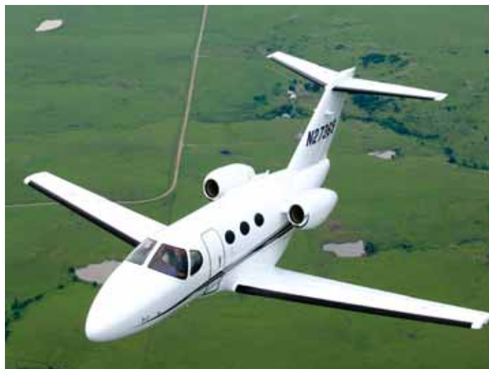
The Cessna Citation Mustang, certification of which is envisioned for later this year, uses Pratt & Whitney Canada PW615F engines for an anticipated cruise speed of 340 knot and maximum operating altitude of 41,000 ft.
