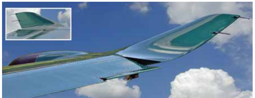
Enhancements for the Pilatus PC-12 include LED lighting (interior and exterior), new crew seats, and new winglets.
