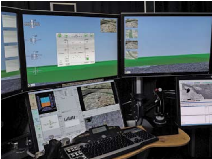
Raytheon's Universal Control System (UCS) features a wrap-around display and dynamic picture-in-picture airspace and weather overlays, live target markers, and digital terrain elevation data.
