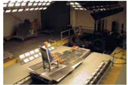
MTS's horizontal acceleration crash simulator will enhance NIAR's ability to test and certify aircraft components under dynamic impact conditions.
