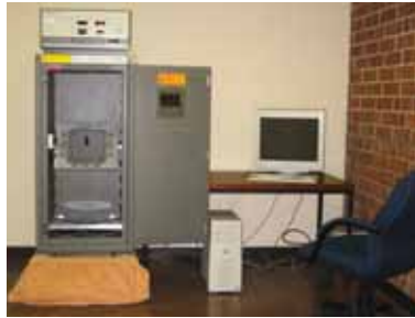
Shown is the Digitome VXI-500 digital x-ray system, a non-mobile version of the device used by NASA to test for defects in a shuttle wing.
