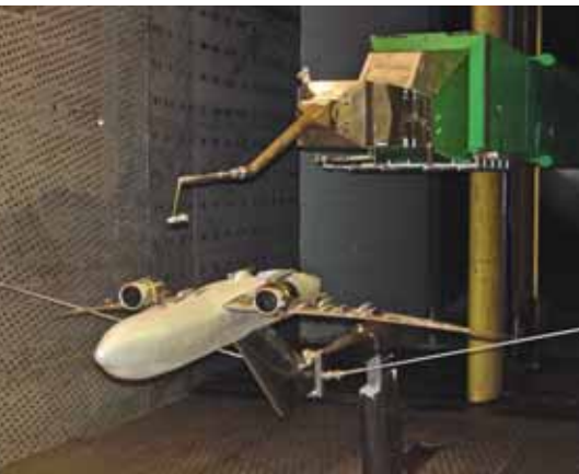
Wind-tunnel tests for separation of weapons from the P-8A aircraft were done with a 6.4% scale model.
