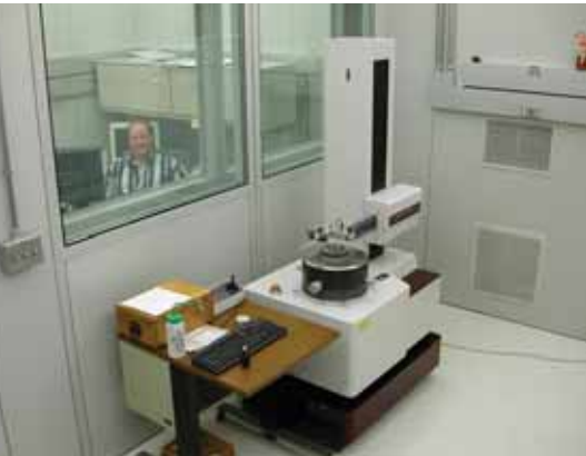
Mitutoyo claims its RA-H5000AS/AH provides the most accurate roundness measurement in the world.
