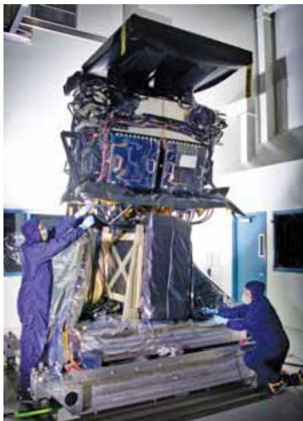
Final preparations are made before thermal vacuum testing is conducted on the payload of the first Space-Based Infrared System geosynchronous-orbit satellite.
