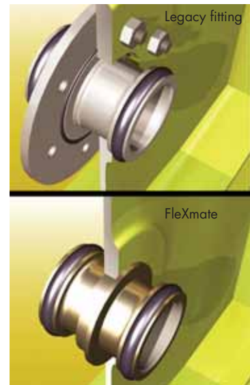
Unlike legacy fittings, FlexMate parts can be cold-expanded into place without the need for satellite holes, a thick pad-up, or complex assembly.
