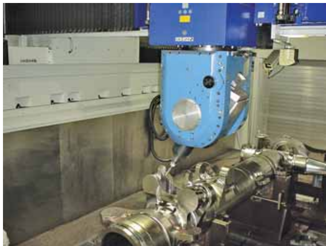
The new high-speed machining cells used by Goodrich split profiling into separate roughing and finishing operations.
