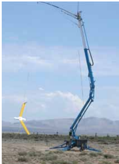
Following a successful net-centric technology demonstration at White Sands Missile Range, NM, Boeing's ScanEagle UAV is retrieved with a patented "Skyhook" system in which the UAV catches a rope hanging from a 50-ft high pole. (Photo courtesy of White Sands Missile Range)
