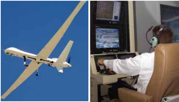
The General Atomics Aeronautical Systems Altair remotely operated aircraft flew a series of climatic and environmental monitoring missions for NOAA and NASA this spring. A pilot for General Atomics guides the UAV from a ground control station using both visual and telemetered data. (All photos courtesy of Tom Tschida)
