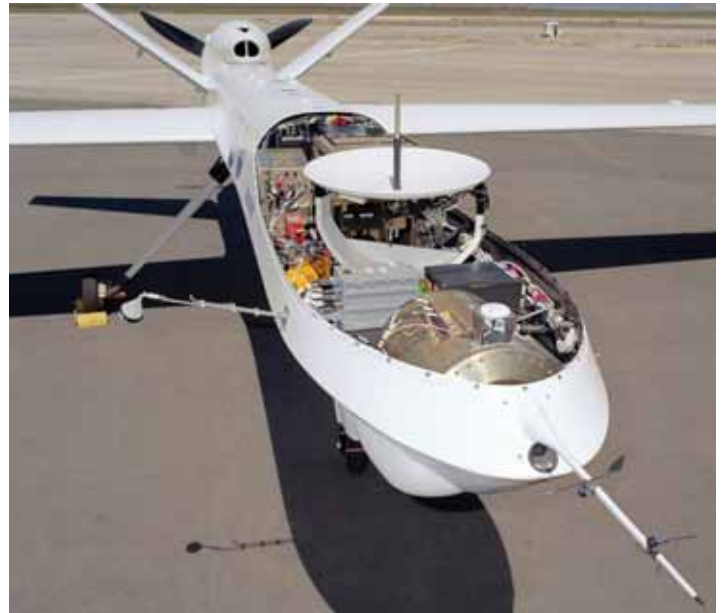
A satellite antenna, electro-optical/infrared and ocean color sensors (front) were among payloads installed on the Altair for the NOAA-NASA UAV flight demonstration.
