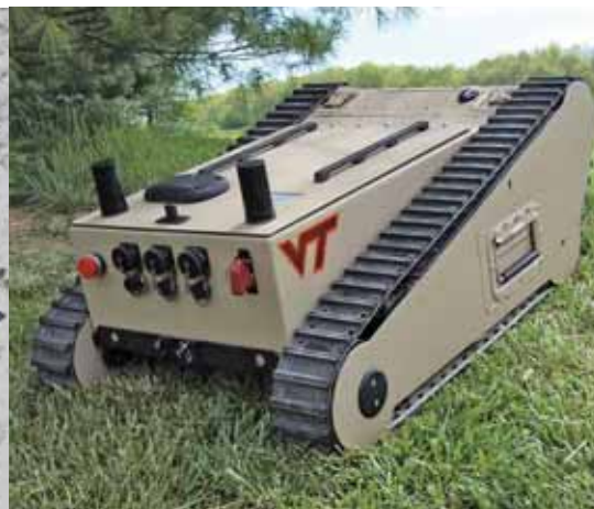
Among the surveillance robots used in the recent JAUS experiment were Harris Corp.'s ADAM (left), which uses Applied Perception's JAUS software suite, and Virginia Tech's Matilda, which was retrofitted for JAUS compliance.
