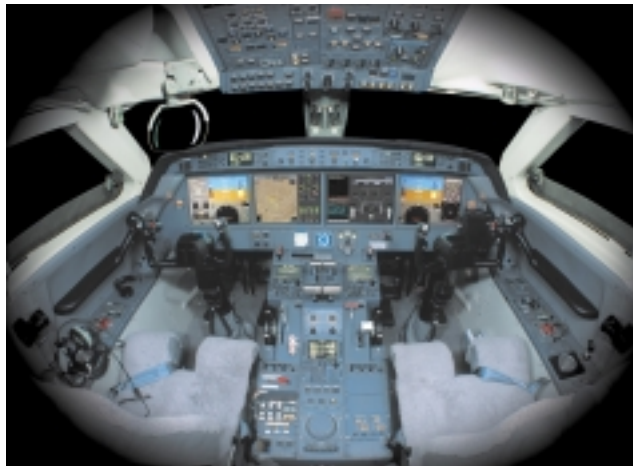
The G350 incorporates Gulfstream's PlaneView flight deck with four 14-in liquid-crystal displays in landscape format for improved pilot situational awareness and reduced workload.
