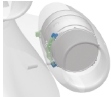
The integrated engine mount system (isolators, yokes, and associated hardware), supplied by Lord Corp., uses titanium in place of stainless steel to help reduce the system's mass by more than 25 kg compared to the original design.
