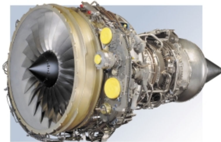
Rated at 18,500 lb of thrust, the GE CF34-10E turbofan engine powers the regional aircraft.
