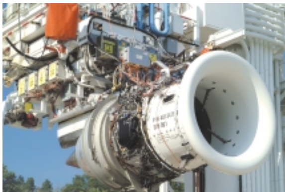
Performance testing of a CF34-10E engine at GE's outdoor test operation near Peebles, OH.
