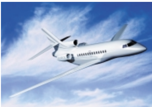
Powered by three Pratt & Whitney Canada PW307A engines, each producing 7500 lb of thermo takeoff thrust, the Falcon 7X long-range business jet from Dassault Aviation will have a range of 5700 nmi.
