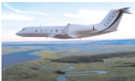
The mid-range Gulfstream G350 business jet is similar in design to the long-range G450 but has fewer standard features and a maximum range that is 550 nmi shorter.
