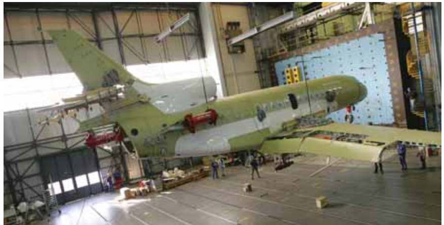
A Falcon 7X test airframe has been undergoing static and fatigue testing since March at the Toulouse Aeronautical Test Center. The airframe has been built as a standard airframe but without most of its internal systems that are not a factor during fatigue testing.
