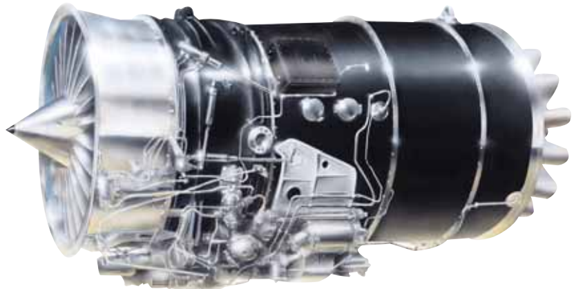
The G450 is powered by two Rolls-Royce Tay 611-8C engines improved specifically for the jet. Performance improvements have been made in the fan, the high-pressure turbine, and the bypass/core mixer. The Gulfstream G350, expected to enter service later this year, also is powered by the Tay 611-8C.
