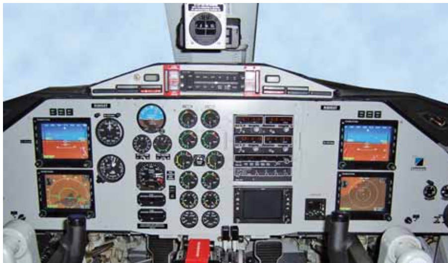
The Chelton Flight Systems FlightLogic Synthetic Vision Electronic Flight Instrumentation System recently was installed in an M28 SkyTruck by Landmark Aviation.
