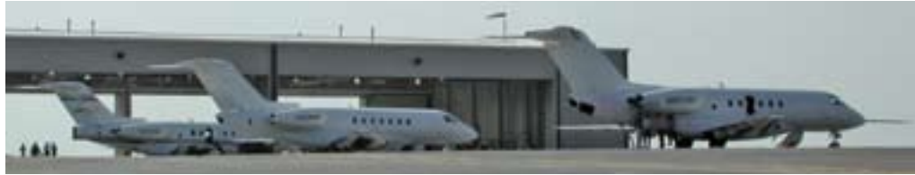
Three Hawker 4000 test articles await flight on the ramp at Beech Field in Wichita, KS. The composite-fuselage plane is powered by two Pratt & Whitney PW308A engines, each delivering 6900 lb of thrust for a maximum cruise speed of Mach .84
