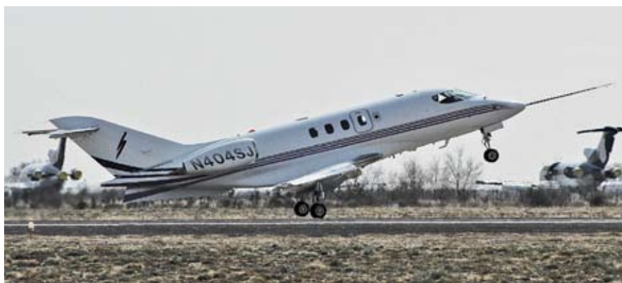
Extreme pitch is not uncommon on takeoff for the SJ30, requiring Sino Swearingen flight-test engineers to conduct VMU testing more common on transport category aircraft.
