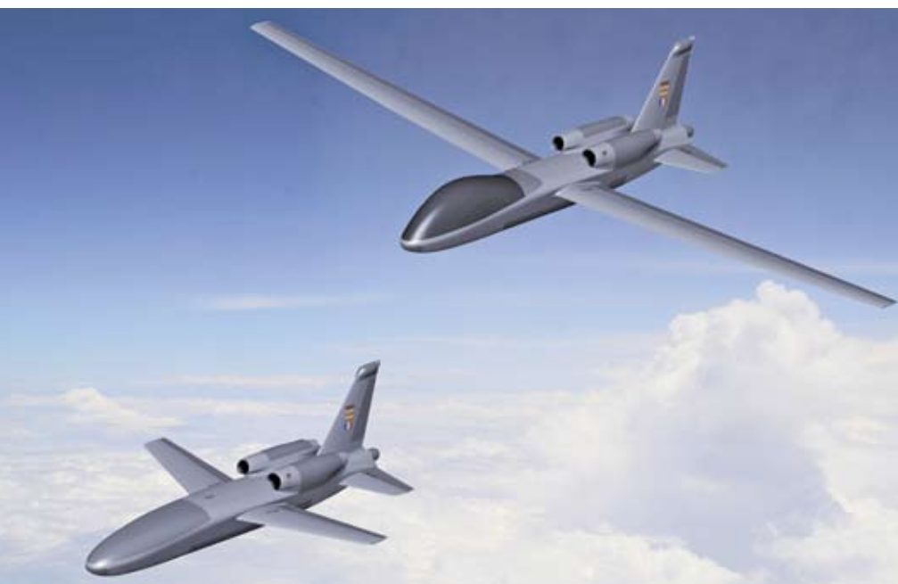
Different wing configurations are envisioned for EADS' modular UAV.
