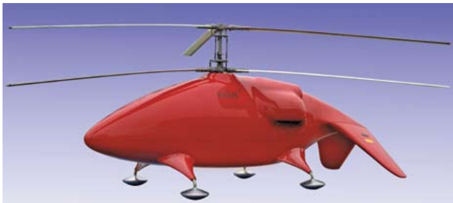
SHARC—EADS' short-range VTOL system for small ship and nonmilitary applications—has a coaxial rotary wing configuration. Payload is up to 60 kg.
