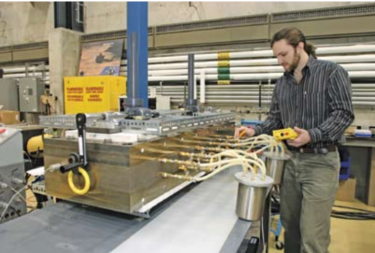
A modular mold was used by NRC Aerospace to fabricate composite rib chords.
