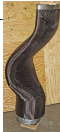
The braided duct preform awaits the VaRTM resin infusion process.
