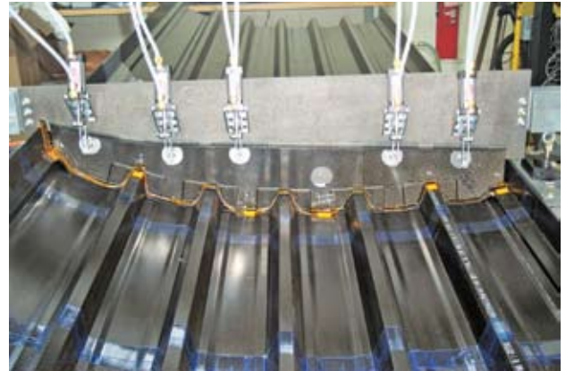
Thermocouples are installed on the bonding fixture for temperature control.
