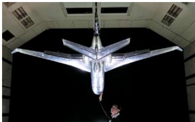
Wind-tunnel testing is another key tool for proving out the Falcon 7X.
