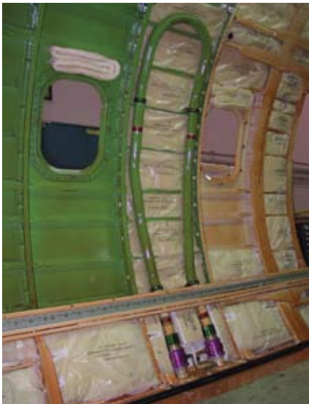
Wolfbend technology is used throughout the Bombardier RJ700 regional jet for fuel supply lines (top two photos) and fuel vent lines (bottom).
