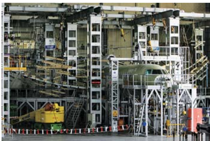
The Falcon 7X's wings are pulled up as much as 2.5 m at the tips as part of the plane's static and fatigue testing regime.
