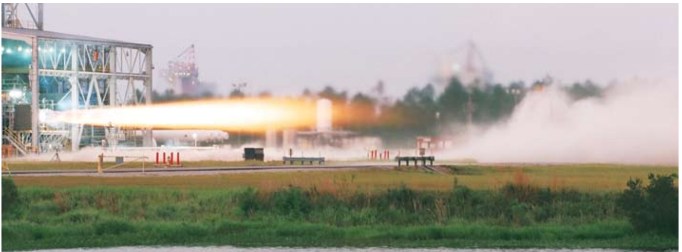
The IPD engine reached steady-state 100% operation—the first U.S. demonstration of the full-flow staged-combustion cycle.
