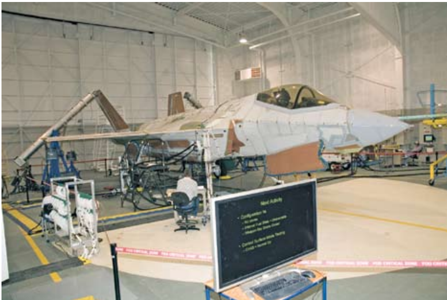
Ground-vibration testing for the F-35 was completed earlier this year.
