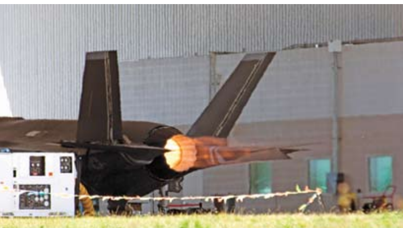
The first series of engine runs in the F-35 took place in late summer. The aircraft is shown here with its afterburner on.
