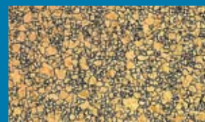
Figure 2: Uniform grain structure of Brush Wellman's Omega-processed copper beryllium
