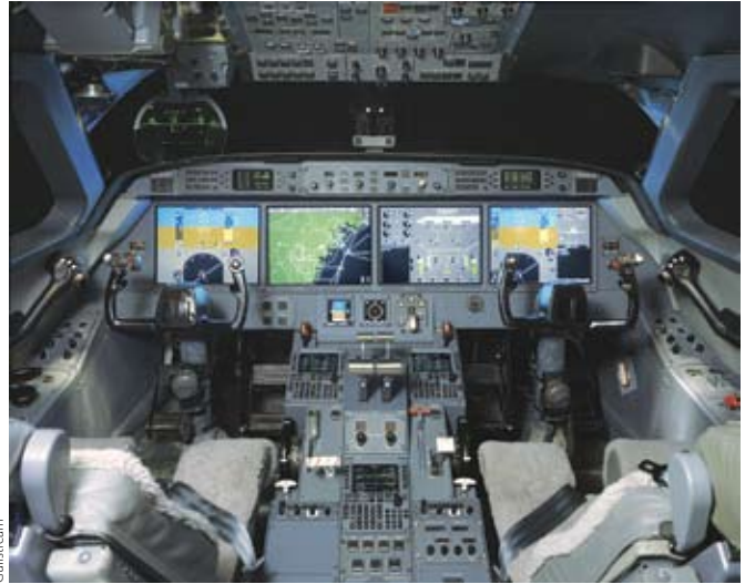
Gulfstream's PlaneView cockpit configuration with four 14-in LCD displays is based on modular avionics architecture from either Honeywell (shown) or Rockwell Collins.
