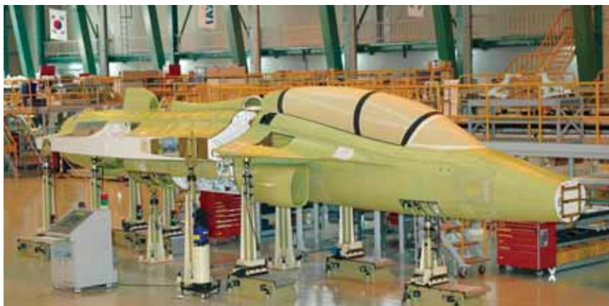
KAI has reached final assembly of the first T-50 supersonic trainer, which was developed by KAI for the Republic of Korea Air Force, with help from Lockheed Martin for the avionics system, flight-control system, and wings.
