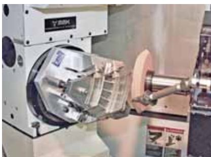
Advanced grinding techniques of aerospace engine turbine blades and nozzle guide vanes is claimed to be saving time and money up and down the aerospace supply chain.
