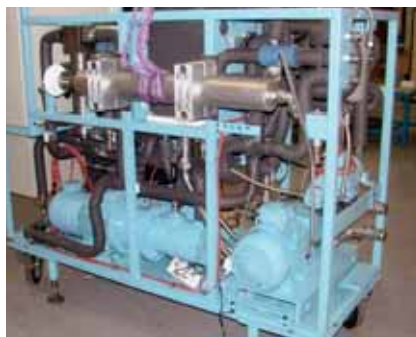
WYKO's hydraulic power pack for the test program of the V-22 Osprey's retractable flight refueling probe was used to determine the system's ability to deliver military-grade oil at high pressure over a temperature range of -55 to +145^{\circ}\text{C} .
