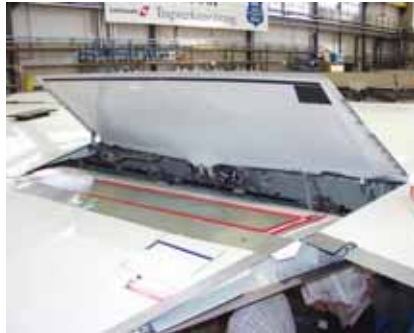
The design of Airbus' weight-saving spoiler involves resin being injected into carbon fiber dry fabric pre-forms. The technology could be used for other, larger structures.
