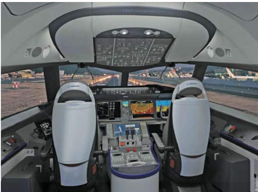
Boeing's involvement in the development of the SAE Aerospace Recommended Practice 5056, Flight Crew Interface Considerations in the Flight Deck Design Process, ensures that controls in the 787 Dreamliner cockpit (shown) will be intuitive and easy to use.
