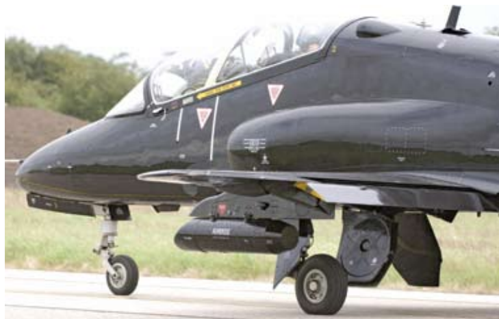
The modified BAE Systems Hawk used for research and development work on the Advanced Structural Health Monitoring System being developed toward the ideal of a totally self-inspecting aircraft.
