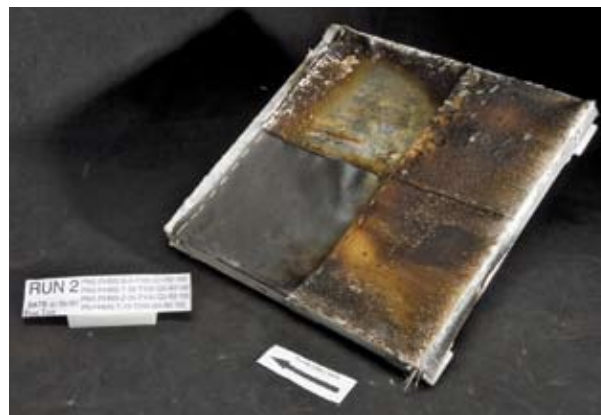
Andrews Space has developed and tested new materials to enable advanced thermal protection systems (TPS) for non-rigid aero surfaces. Shown is the result of a coupon sample test of the TPS materials.
