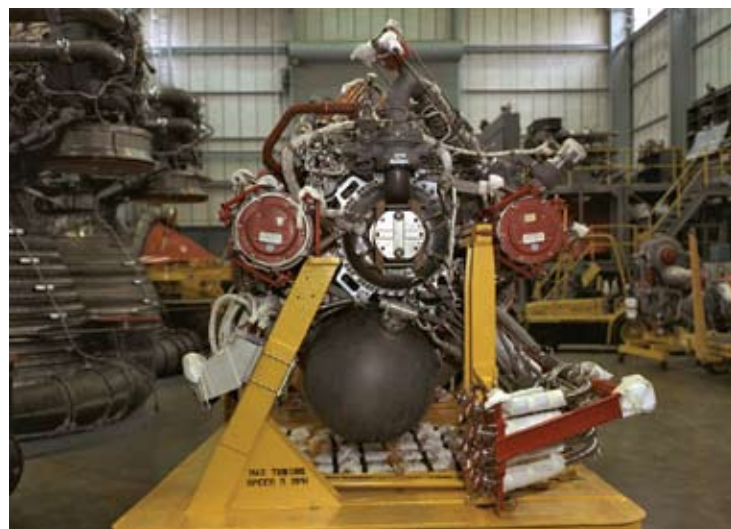
An original J-2 engine for the Saturn V undergoes processing at NASA's Marshall Space Flight Center in 1965. The Saturn V, like key hardware and components of the Ares launch vehicles, was designed, developed, and tested by Marshall Center engineers.
