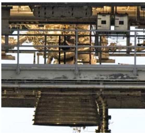
A J-2 engine awaits testing on the A-1 Test Stand at SSC. NASA is testing the engine's powerpack—a gas generator and turbopumps that perform the rocket engine's major pumping and combustion work. The engine is being studied anew by NASA rocket scientists building the engines that will power the next generation of launch vehicles, the Ares I and Ares V, and carry humans to the moon.
