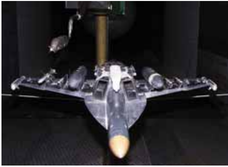
The 10% EA-18G model in the AEDC 16-ft transonic wind tunnel is configured with ALQ-218 pods on the wing tips, an AGM-88 HARM on the left outboard station, 480-gal fuel tanks on the inboard stations, and an ALQ-99 low-band pod on the centerline station.
