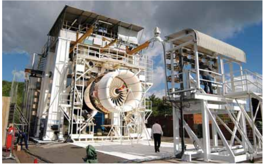
High-temperature materials will be one area of focus for Rolls-Royce and Singapore's A*STAR organization. Here, preparations are made for an engine blade-off test.
