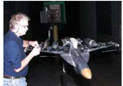
Arnold Engineering Development Center (AEDC) Lead Outside Machinist Larry Towry inspects the 10% scale EA-18G parent aircraft and captive trajectory system store models in the wind tunnel.
