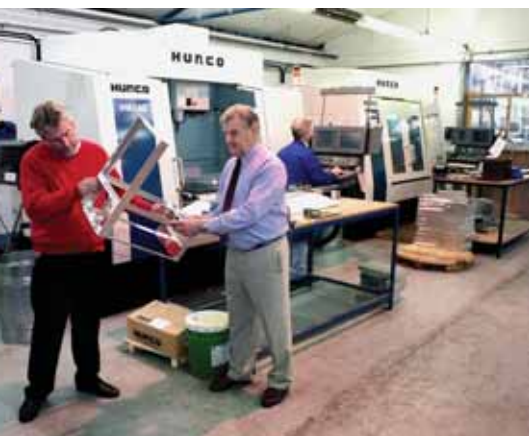
Ken Metcalfe (right) and Aerolux Engineering Manager Glen McQuire check an aluminum frame for an aircraft galley refrigerator that has machined components.
