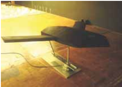
Wind-tunnel test of the Santos flapless research vehicle, which is the result of a five-year project that will cover key aspects and technologies of the next-generation UAV.
