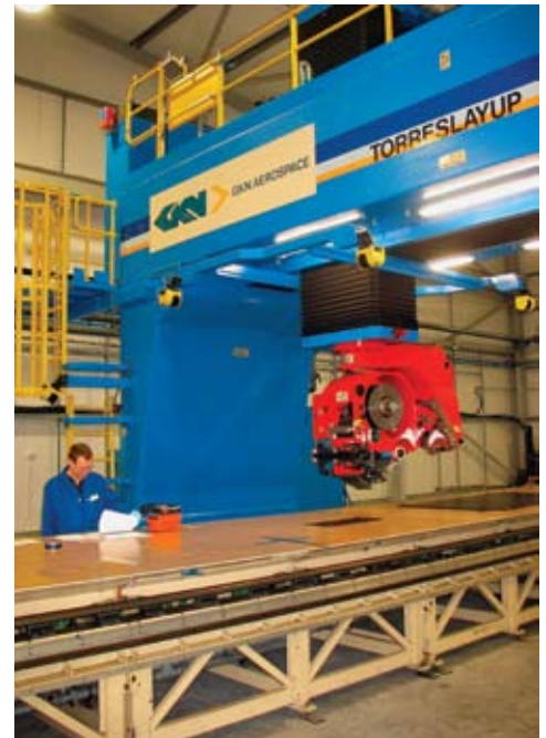
For winglet manufacture, GKN uses an automated tape-laying machine similar to the one shown, which is used to make the Airbus A400M composite wing spar.
