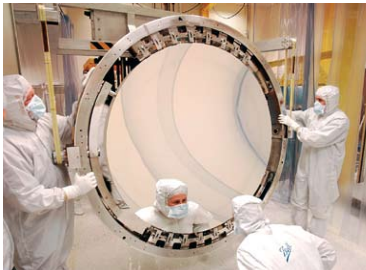
Ball Aerospace's completion of the Kepler primary mirror's coating culminates a four-year development program to design and build a large, lightweight mirror for use in space.
