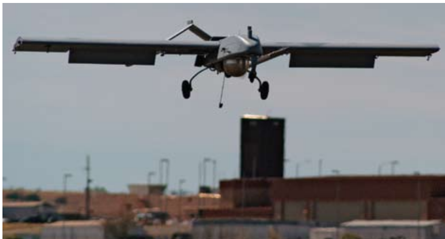
Both the German-built Luna UAV and the Shadow tactical unmanned air system (shown) have autonomous navigation and control systems from Athena Technologies.
