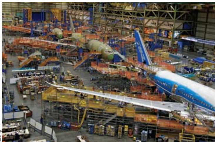
This was the 787's state of production in early December. The first unit (dedicated to flight testing) was nearing completion while the two ground-test units were undergoing major assembly.
