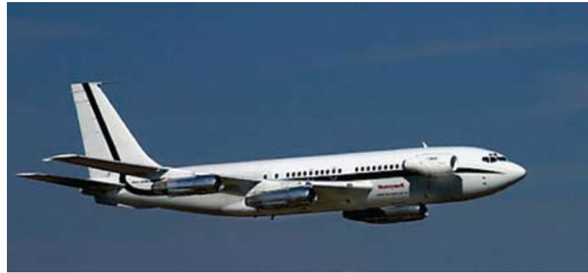
This Boeing 720 is a good, stable testbed for the size of turbofan engines that Honeywell produces, according to Mark Steele, Manager of Advanced Engines, APU, Commercial Propulsion Performance, Honeywell. The engine under test in this photo is the one attached to the front fuselage.
