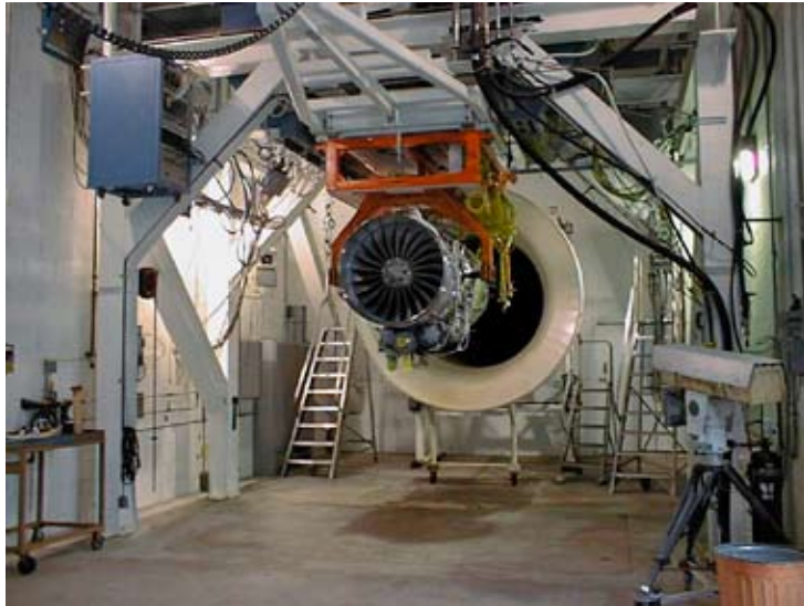
Between actual flights and this cell located in Phoenix, Honeywell can run all of the engine rating tests required by customers, said Steele. Temperature is not controlled in the cell, but Honeywell engineers can refer the engine data to temperatures defined in ARP210.
