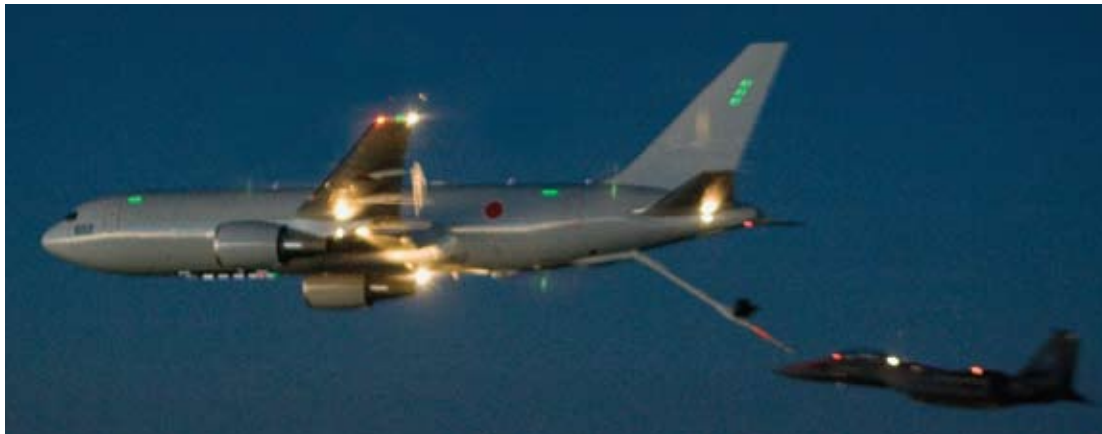
A Boeing KC-767, one of two tankers scheduled for delivery to Japan this quarter, prepares to transfer fuel to an F-15E over the skies of Missouri in late January. It was the first nighttime refueling ever accomplished on a KC-767, which features a remote vision system for the boom operator.
