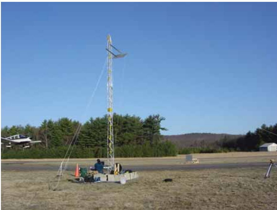
WPI's wake-turbulence detector uses reflectors on a tower and on the opposite side of the runway to direct high-frequency sound across a closed path. Vortices from an airplane are detected by sensing variations in the speed of the sound waves.
