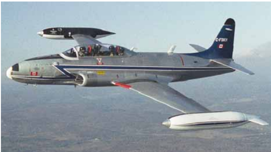
The National Research Council of Canada is outfitting a Lockheed T-33 to replace its Dassault Falcon 20 for more rugged wake studies.
