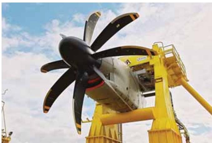
Ratier-Figeac's eight-bladed composite propeller was designed specifically to handle the high-power output of the 11,000-hp EPI engines that will be powering the A400M from Airbus Military.
