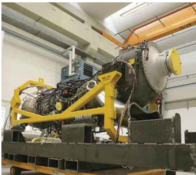
Airbus claims that EPI's three-shaft, high-performance turbine TP400-D6 is "the most powerful turboprop powerplant in the Western world."
