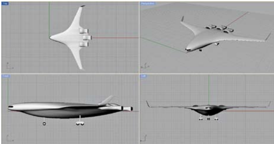
The concept design for the Cambridge-MIT Silent Aircraft Initiative is based on a blended-wing configuration that would emit noise nearly imperceptible outside the perimeter of an urban airport.
