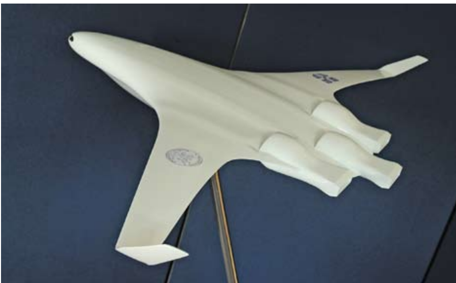
An airliner for 2030? The Cambridge-MIT Institute's concept for the SAI features an “all-lifting” design, producing lift on the center body as well as the wings.
