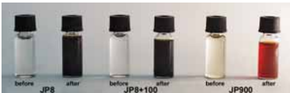
Researchers at Penn State have developed a jet fuel designated JP900 that is derived from bituminous coal and meets or exceeds almost all specifications for JP8 and Jet A.
