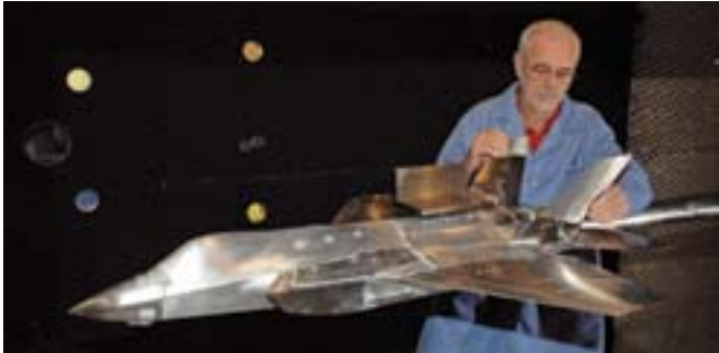
ATA Outside Machinist Carey Wofford checks the movement of the vertical stabilizers of a F-35 test article prior to resuming the aerodynamics test.
