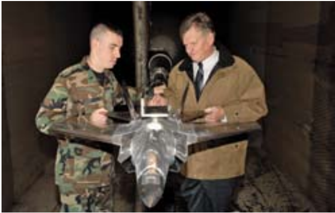
First Lt. Ezra Caplan and ATA Senior Project Engineer Charlie Smith examine a 12% scale model of the F-35C during a break in the final pre-production aerodynamics testing done on all F-35 variants.
