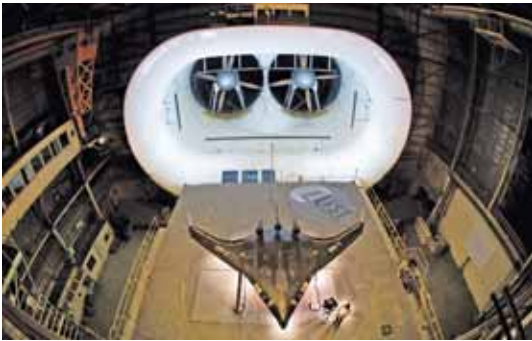
Wind-tunnel testing on the X-48B Ship No. 1 began on April 7 at the Langley Full-Scale Tunnel. After testing is complete, it is scheduled to be shipped to the Dryden Flight Research Center to serve as a backup to Ship No. 2, which will be used for flight testing later this year.
