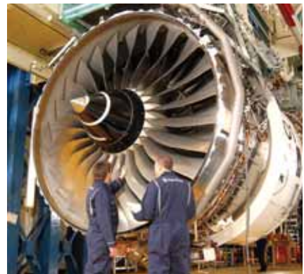
Four Rolls-Royce Trent 900 engines took the first Airbus A380 into the air.
