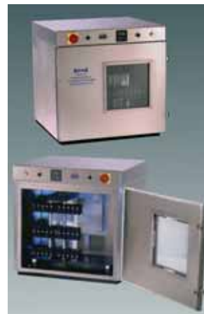
The Benz DFT2100 DeMattia can be pre-set to as many as 10,000,000 cycles and then digitally display either the number of cycles remaining in the test or the number that have been completed.
