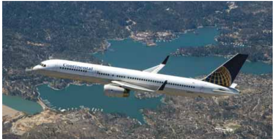
Continental Airlines is the first carrier to fly a Boeing 757-200 aircraft with blended winglets, which are said to increase fuel efficiency and range.
