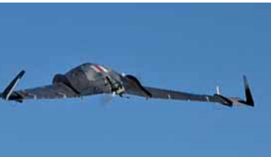
The Inventus E features a cruise speed of 44 mph (battery life 120 min), maximum speed of 85 mph (battery life 20 min), range of 90 mi, and altitude of up to 10,000 ft.
