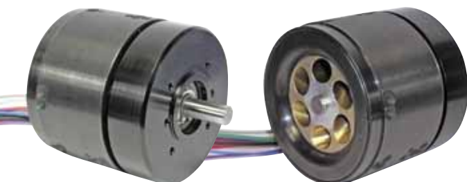
The inside and outside surfaces of the ThinGap coil used in the Inventus E are exposed to moving air inherently pumped into the gap by the rotor, allowing the use of more current without overheating the motor. There are no laminations or iron core in the ThinGap motor.
