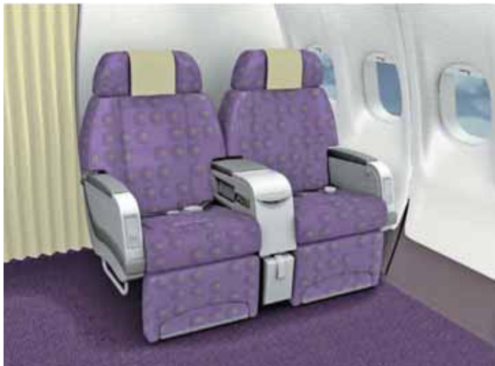
Airline seats incorporating GE Plastics' Ultem resin are claimed to protect aircraft cabin fabrics and carpet better than traditional textiles and non-woven types.
