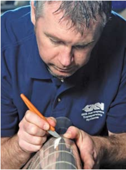
Surface preparation is done by a GKN Aerospace specialist prior to application of an electro-thermal heating element.
