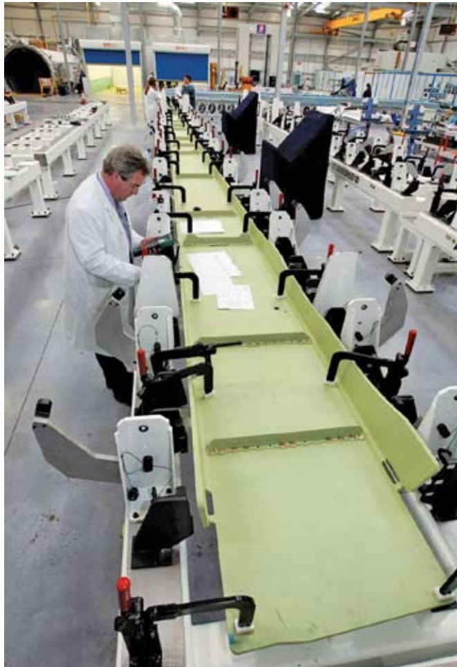
The 20-m-long, all-composite wing spar for the Airbus A400M military airlifter is being completed by GKN Aerospace.
