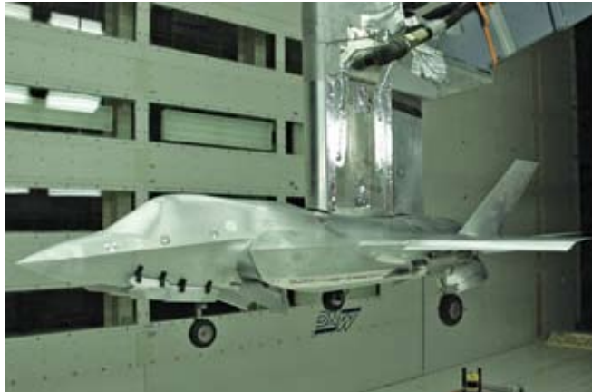
A 12% jet effects scale model of the STOVL F-35 Joint Strike Fighter in the DNW Large Low-speed Facility. Particle image velocimetry is used by DNW for ground visualization of the exhaust flow of the aircraft and to give quantitative information about flow velocity.
