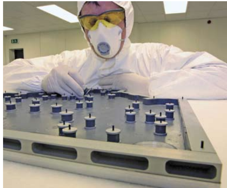
Prodrive has built composite panels for Surrey Satellite Technology for use in space applications.
