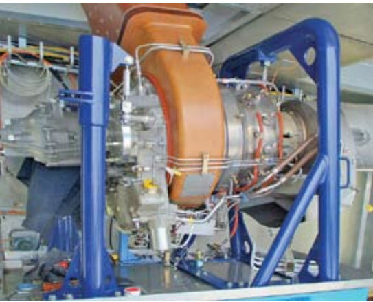
Fewer suppliers were selected for the 787 program, but those that were had more responsibility than those on previous programs. Hamilton Sundstrand (whose auxiliary power unit for the 787 is shown above, on a test stand) has a large role in electrical power generation and distribution on the new airplane.
