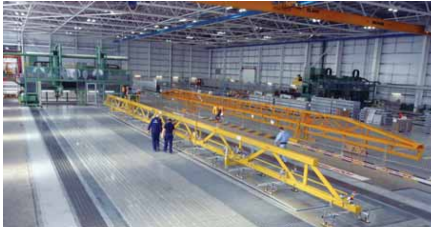
Checking a billet on the bed of the A380 wing skin milling machine at Airbus UK.
