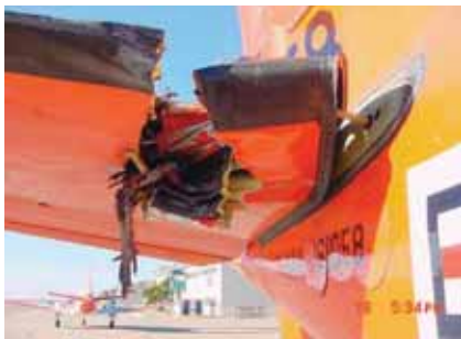
Bird-strike damage can endanger aircraft, and a consortium of industry and academic institutions is involved in finding ways to improve testing methods.
