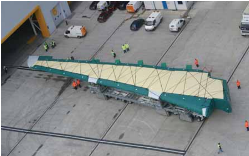
An Airbus A380 wing leaves Airbus UK's Broughton factory en route for Toulouse and final assembly.
