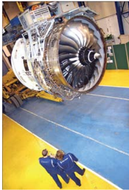
Research into cooling the "hot end" of gas turbines is to be carried out by Rolls-Royce and Karlsruhe University. Pictured is the Rolls-Royce Trent 1000 for the Boeing 787.
