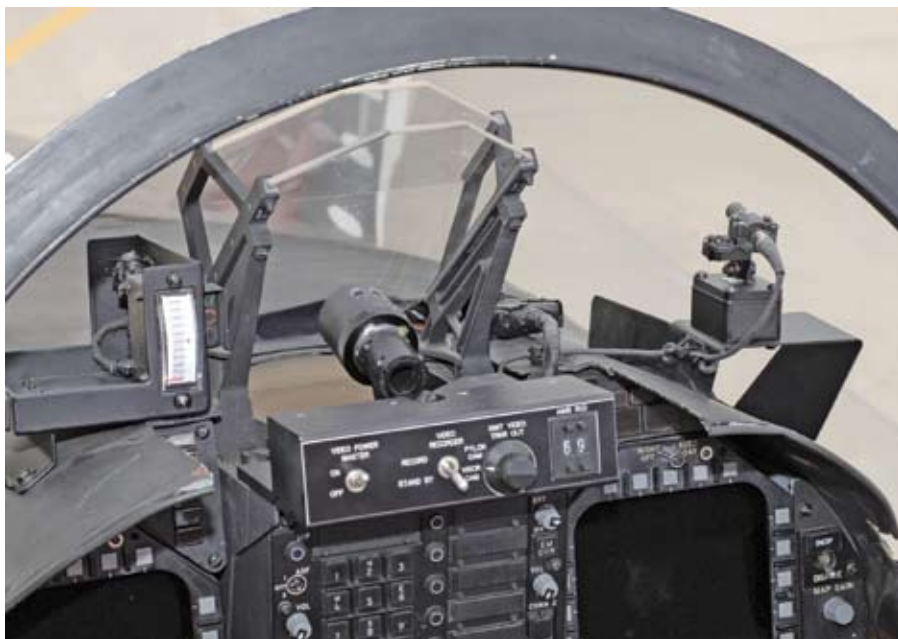
The HUD and video camera setup in the cockpit of the AARD F/A-18. A pilot was onboard the aircraft during the test for safety purposes.
