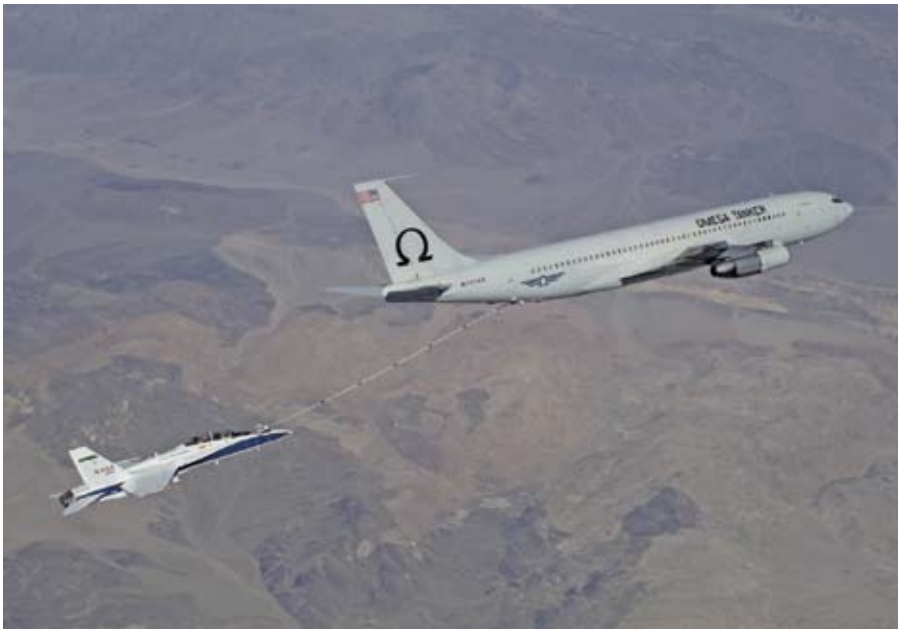
An F/A-18 that was configured to operate as an unmanned test bed is shown behind a 707 from Omega Air Refueling Services during an Autonomous Airborne Refueling Demonstration (AARD) flight.
