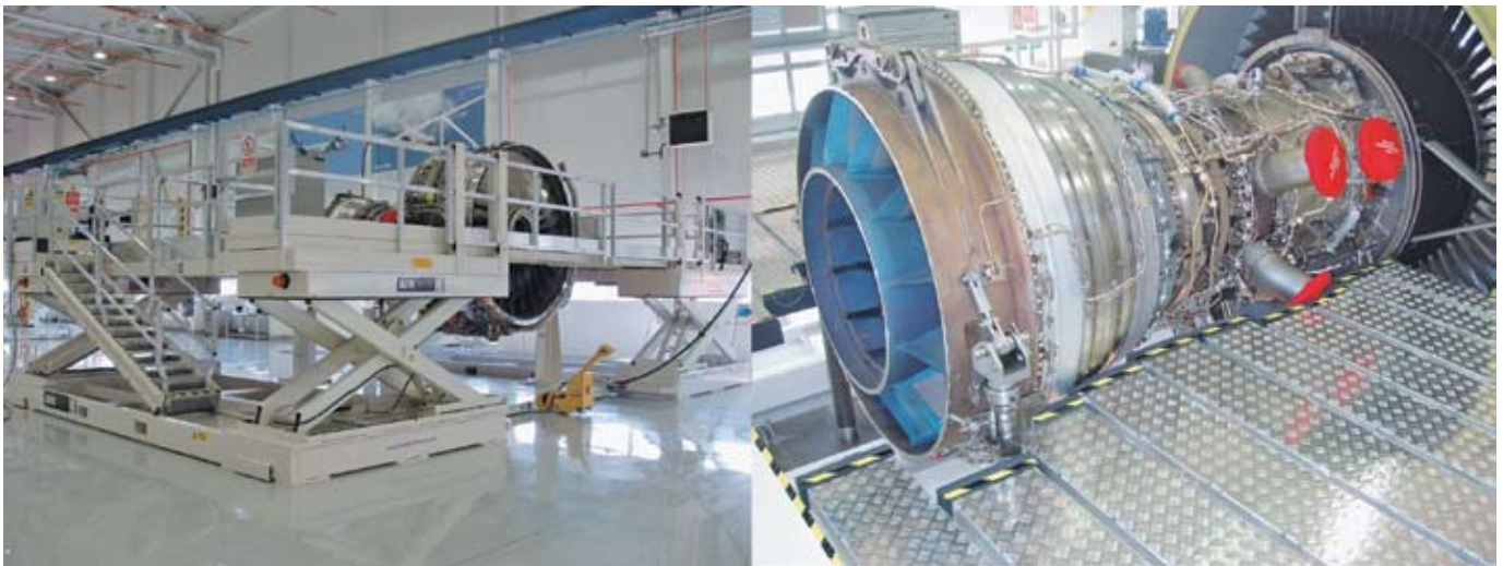
The AIRdeck intelligent access platform from Planet Platforms was initially developed specifically for the final inspection process of Rolls-Royce's 500, 700, 800, and 900 Trent engines.
