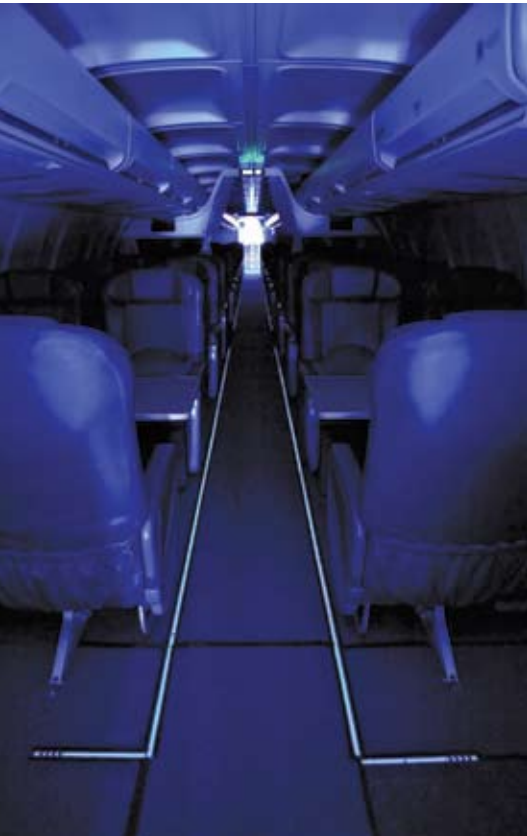
STG's latest ColorMatch floorpath system has been designed to blend with airline cabin decor.
