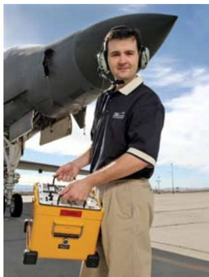
Designed to test electronic-warfare capabilities, EDO's system simulates RF signals generated by anti-aircraft weapons.
