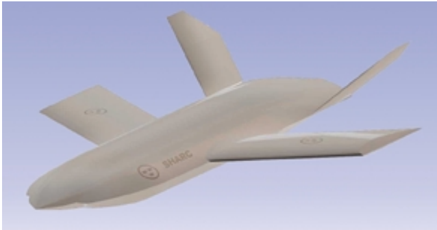
Saab Aerospace's UAV, called SHARC, measures 10 m long and has a wingspan of 8 m.
