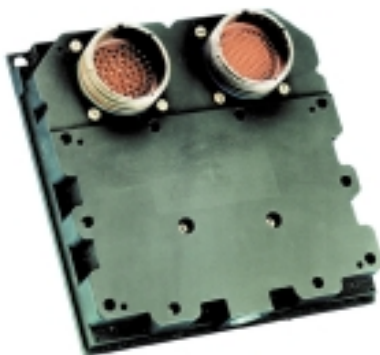
Smiths Industries Aerospace developed a remote input/output unit for the Lockheed Martin JSF vehicle management system.
