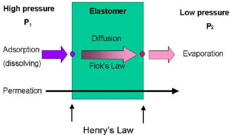
Combining Henry's and Fick's laws gives us the general gas permeation equation for permeation through a parallel faced membrane :-
