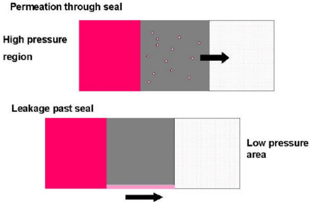
Once stress relaxation and set have happened due to a long period of use at high temperature, leakage *past* the seal may occur. This is most likely to happen during cold cycles when thermal shrinkage exacerbates the effects of set. This leakage will result in an uncontained loss of the refrigerant fluid.
