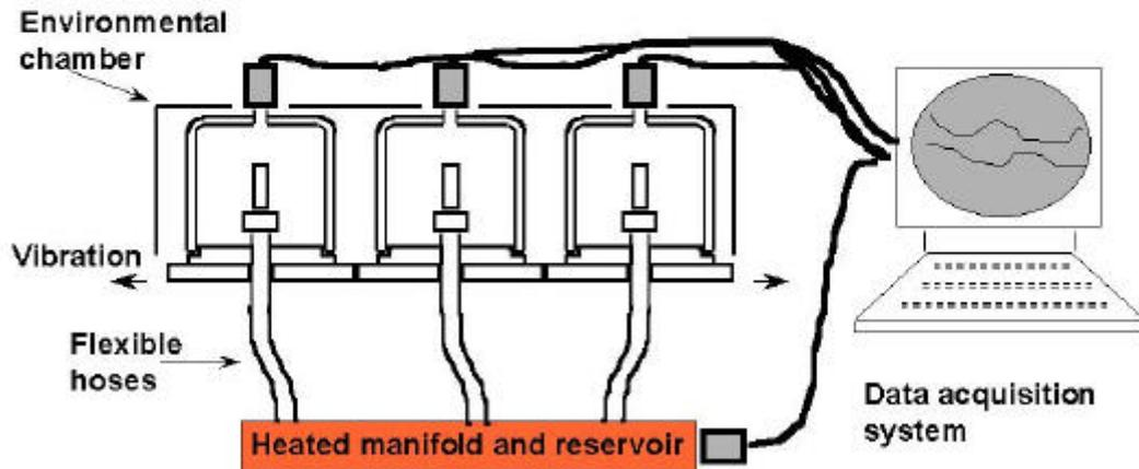
The gas collection cells are contained in a close fitting chamber with heating and cooling facilities. The possible operating envelope of the rig is shown in table 5 below:-
