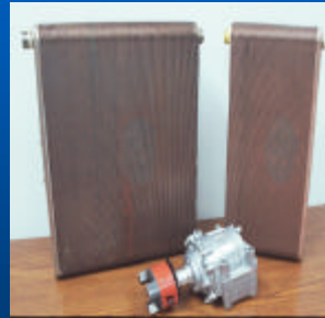
1 st and 2 nd generation Internal Heat Exchangers (compressor shown for scale)
