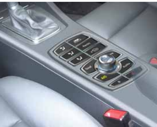
When the air-conditioning function is selected, circulation icons appear on buttons of Preh Automotive's freely programmable button (FPB) concept.
