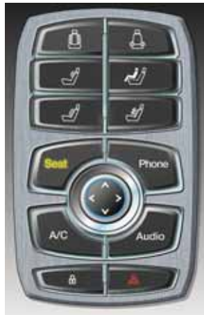
If the seat function is chosen, seat position icons appear on the buttons.
