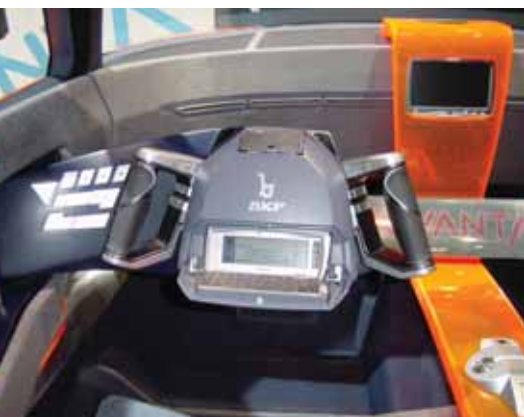
Novanta's human machine interface employs a handle mechanism that is integrated into the driver's door. Once the driver is seated, the mechanism swings from the door to form a controls pod for the driver.
