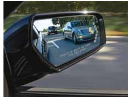
While a vehicle is visible in the rearview mirror, an amber-colored alert indicates that a vehicle is in the blind zone of the right side of the vehicle.
