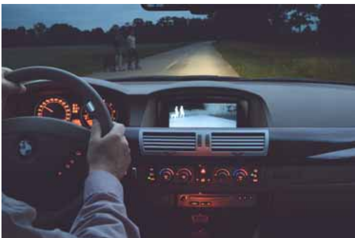
BMW's Night Vision uses far infrared technology developed in conjunction with Autoliv.
