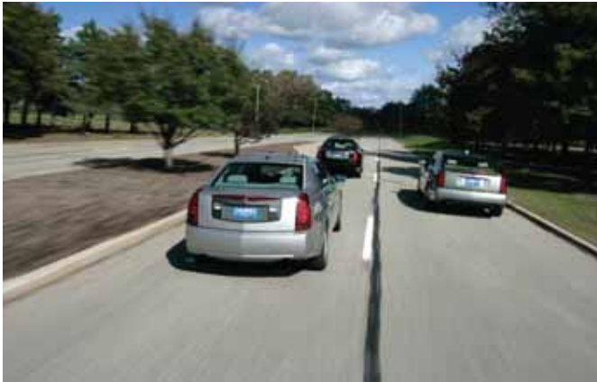
GM vehicles equipped with vehicle-to-vehicle technology can detect the position and movement of other vehicles.
