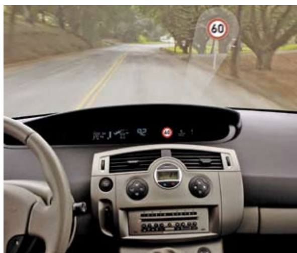
Analog Devices' traffic-sign recognition prototype is based on embedded computing; a single processor accomplishes the task.
