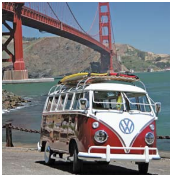
VW's Vickie Chiang was involved in retrofitting a 1964 Microbus with new technologies such as adding flexible solar cells to a roof-rack stowed surfboard. The solar cells provide supplemental power for charging the Microbus.
